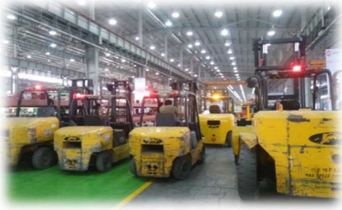
Buzzer and Flasher Light installed on all Fork Lifters and Cranes
