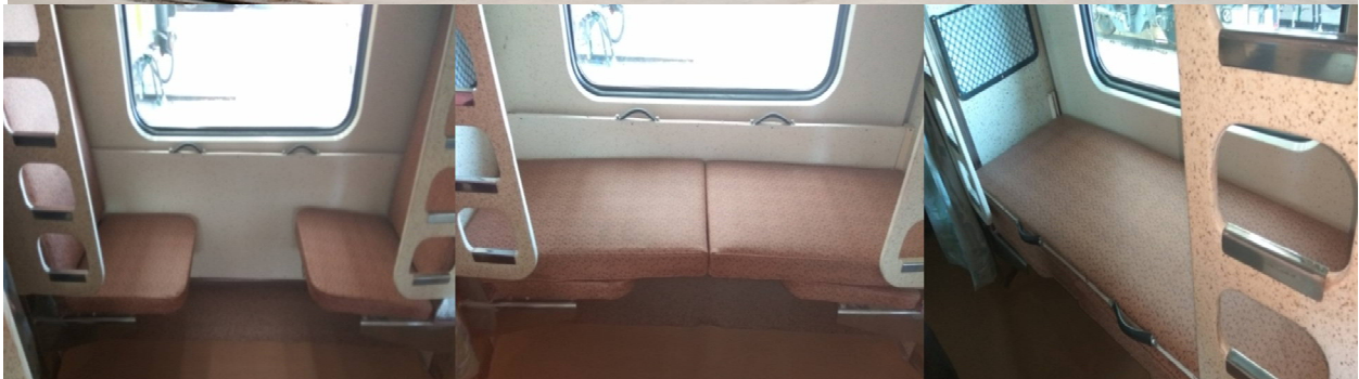
Single piece side lower berth - first time in Indian Railway, introduced in upgraded Humsafar Express
