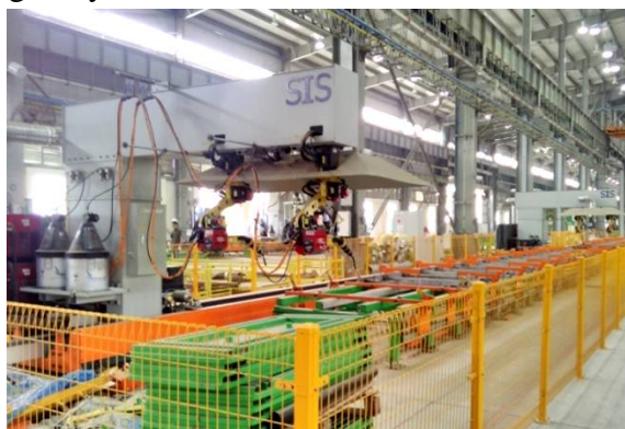
(Automated side wall manufacturing line)
