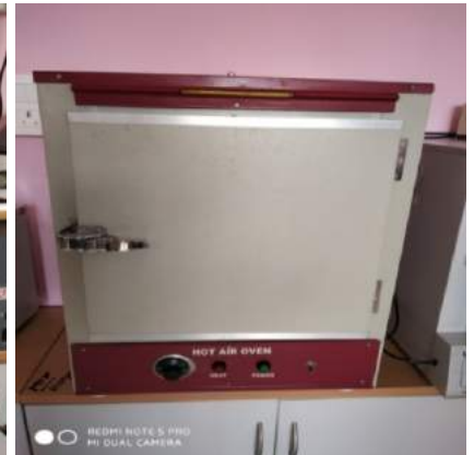
HOT AIR OVEN: For sterilization of Test Tube, Slides, Culture Plates.
