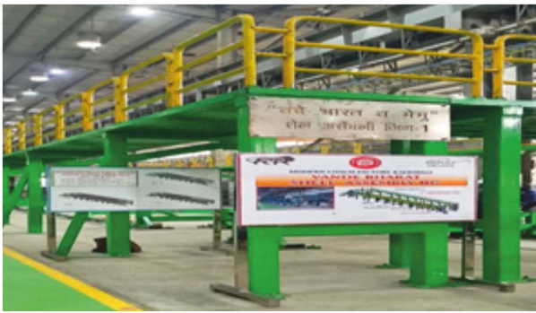
Shell Assembly Jig
